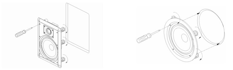
**STEP E.** The final step is to install the grill. The grill fits into the speaker frame recess. Starting at one corner or side, gently press the grill into the recess. Continue around the frame a bit at time. Do not excessively handle the grill. Doing so will dent and/or bend the grill out of shape, thus harming the appearance.
